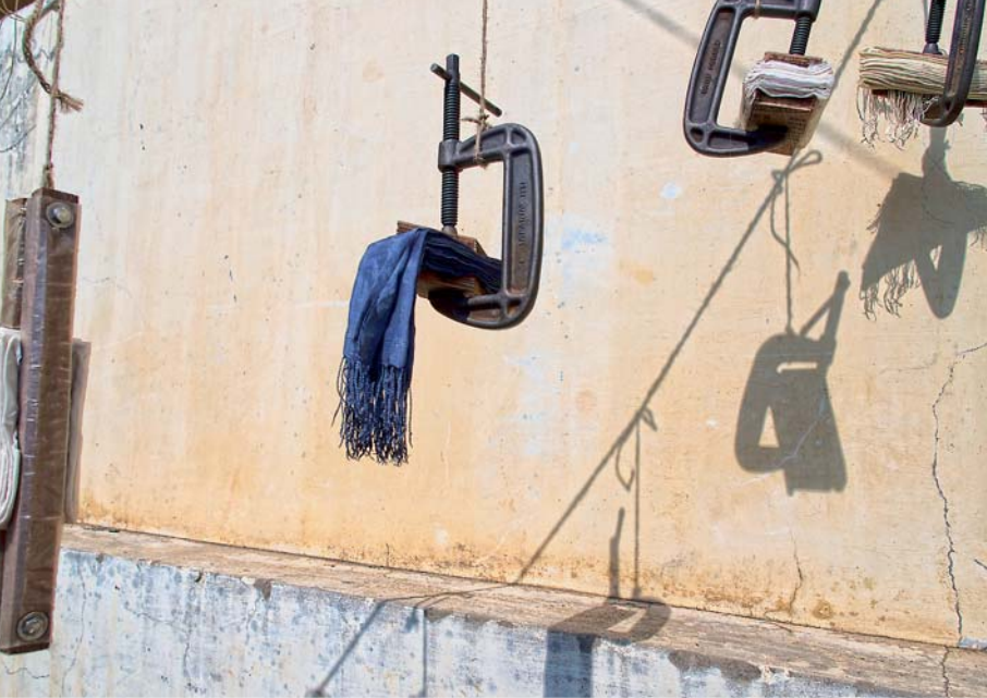
Left: Bhadali village's textile trade is built on a "tie-and-dye" technique. Here, clamps prevent dye from penetrating the compressed parts of the bundled or folded fabric, resulting in brilliant patterns now familiar worldwide, lower.
